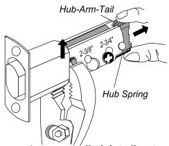
You may also use a slip-joint pliers to push up the Blocking-Pin and hold in position instead of using the fingers. If a pliers is in use, make sure just give enough pressure to hold the Blocking-Pin in up position. Over tightening could damage the latch construction. To set the slip-joint pliers for wider clamping position reduces the clamping pressure.
