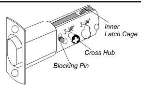
The D400-DF67 UL-Deadbolt is 2-3/8" and 2-3/4" field - convertable. The Deadbolt packed is set for 2-3/8" backset. You may apply the Faceplate furnished onto the Latch Front for installation if 2-3/8" backset is your application.
